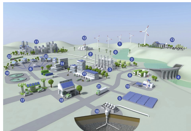
Fig. 9 – Future energy system - WIVA P&G [108]. Energy supply: 1 Wind power plant, 2 Biogas plant, 3 Gas power plant, 4 Hydro power plant, 5 PV power plant; Energy distribution and storage: 6 Regional gas grid with municipal storage, 7 Supra-regional gas grid, 8 Electricity grid, 9 Central electrolysis/methanisation plant, 10 Hydrogen/natural gas storage; Energy use: 11 Smart City and zero-emission public transport, 12 Green industrial processes, 13 Energy-autonomous agriculture and small businesses, 14 Smart buildings, 15 Green intralogistics, 16 Sewage treatment plants, 17 Hydrogen/gas/electric filling station, 18 Energy-autonomous single-family house, 19 Energy-autonomous remote station, 20 Smart village, 21 Zero-emission heavy traffic, 22 Zero-emission rail traffic.
