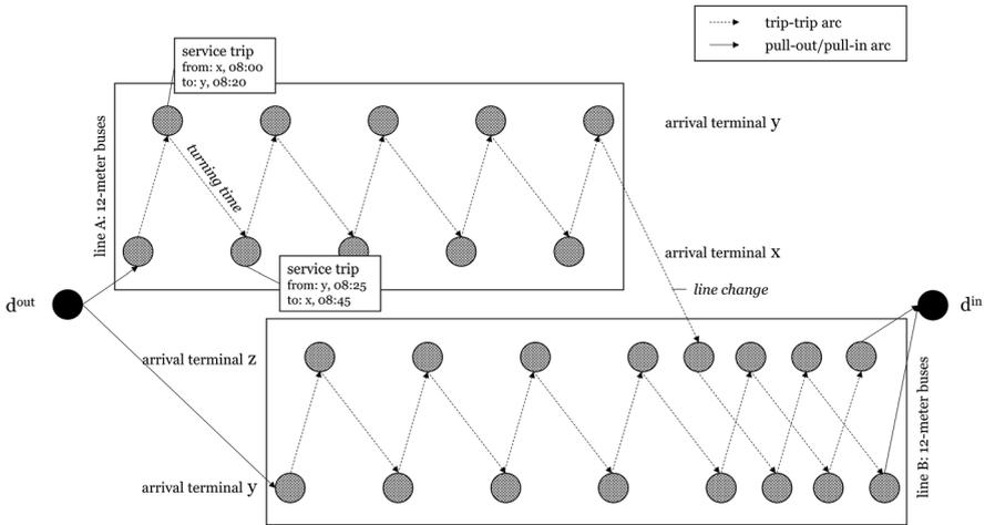
Fig. 3 Solution of a base network
