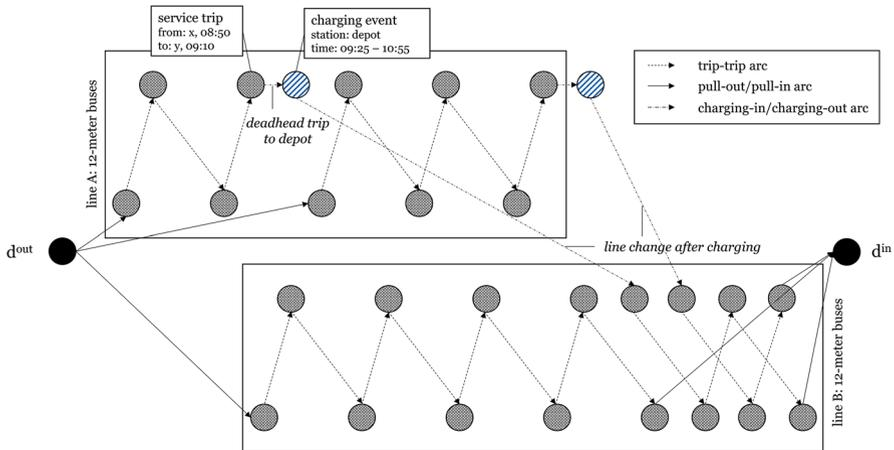
Fig. 5 Solution of an ONC network
