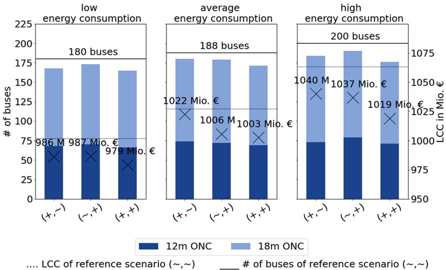
**Fig. 10** Comparison of LCC and fleet composition of ONC networks for different charging factor combinations. Each charging factor combination is signified by a tuple (battery capacity, charging power), which indicates the respective state of battery capacity and charging power. ~ stands for standard factor levels, a + represents an increase in battery capacity or charging power
