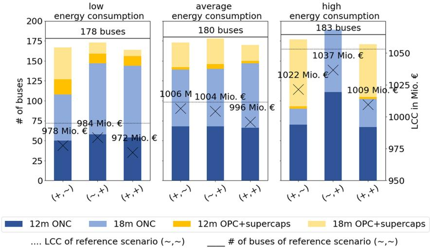
**Fig. 9** Comparison of LCC and fleet composition of the technology mix for different ONC factor combinations. Each charging factor combination is signified by a tuple (battery capacity, charging power), which indicates the respective state of battery capacity and charging power. ~ stands for standard factor levels, a + represents an increase in battery capacity or charging power
